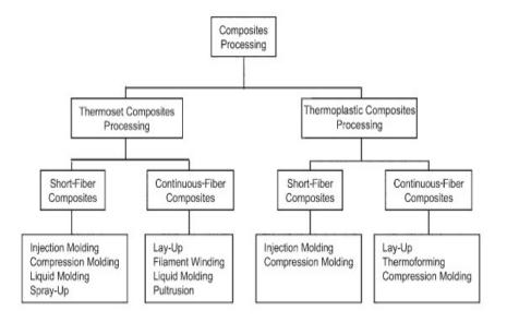
Fig 1.1 Classification of fibre reinforcement processing
