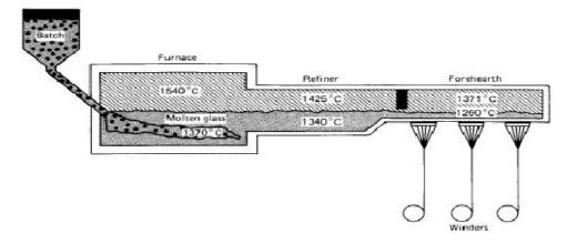
Fig. 3.3: Furnace for glass melting (ASM International, 2001)
