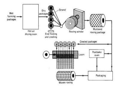
Fig 3.42:- Multi end roving process production (ASM International, 2001)
