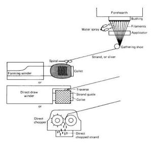
Fig 3.4: Fibre glass forming process (ASM International, 2001)
